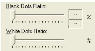
For white pages, use the [Black Dots Ratio] slider bar to specify a degree of accuracy needed to skip blank pages. For black pages, use the [White Dots Ratio] scroll bar to specify a degree of accuracy needed to skip blank pages. The value displayed to the right of the slider bar shows a noise (dots) ratio(\*1). If a scanned page includes dots less than this value, the page is recognized as blank. You can select OFF(- -) or a value from 0.2% to 3.0% (in increments of 0.2%).
