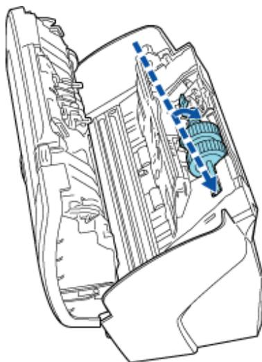
2) Rotate the Pick roller lever in the direction of the arrow.
