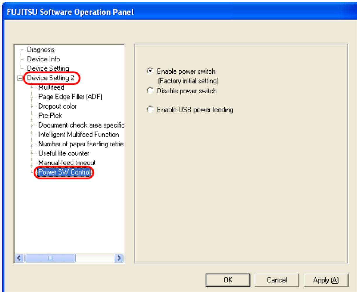
3. To power on/off the scanner by pressing the Power button, select [Enable power switch]. To power on/off the scanner by connecting/disconnecting the AC cable, select [Disable power switch].
