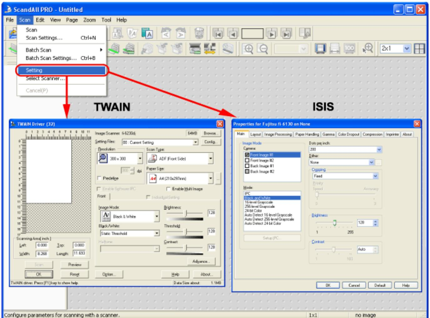
5. In the driver setup dialog box, configure settings for scanning.
