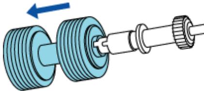
**5. Attach a new Brake roller.**
