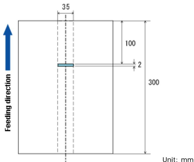
\* Since the detection range (length) is less than the minimum value (5 mm), the Multifeed Detection cannot be performed correctly.
