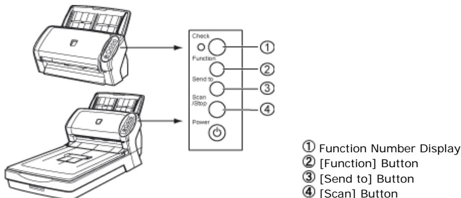
**2. When using this function, press the [Function] button, and then make sure that the function number blinks at shorter intervals before you press the [Scan] button or restart scanning by using the personal computer.**
