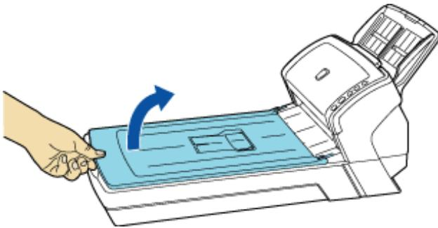
2. Load the document on the document bed with the scanning face down and the top left corner aligned with the reference point (①).
