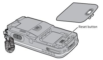
**3** Use the stylus to press the **Reset** button on the back of the CN3.
