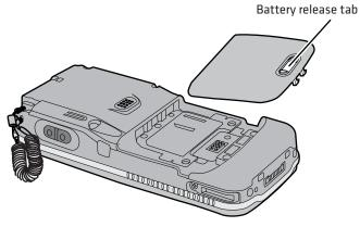
Removing the Battery in a CN3e
