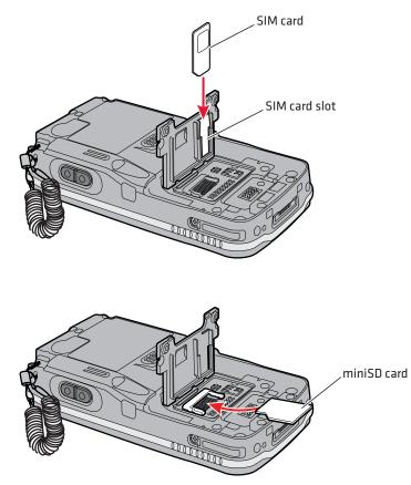
**5** Close the miniSD/SIM card slot door and insert the two screws.
