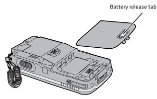
Removing the Battery in a CN3
