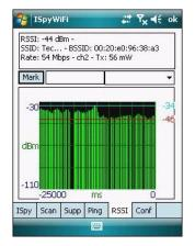
The information box includes the current signal strength, host SSID name, MAC address, data rate, and transmit power.
