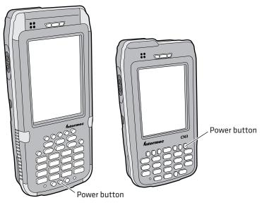
In this lower power mode, the CN3 continues to supply power to all memory, but turns off power to most hardware such as the display. This feature is designed to prolong battery life.
