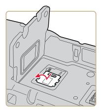
Slide the microSD card door towards the top of the computer to unlock it and open the door.
