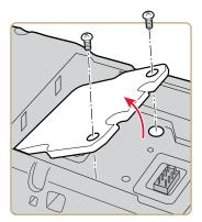
**3** On the CK70, remove the two screws and lift the card access door away from the computer.
