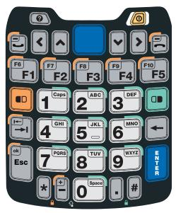
The CK70 comes with either a large alpha or an alphanumeric keypad. The CK71 comes with either a numeric function keypad or an alphanumeric keypad. The computer has an ambient light sensor that detects low light and turns on the keypad backlight. By default, the keypad backlight is enabled in low light conditions. You can disable the keypad backlight to conserve power. Use Intermec Settings to configure the backlight. For help, see "Use Intermec Settings on the Computer" on page 77.
