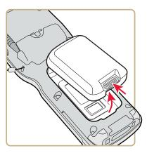
**6** Insert the top end of a fully charged battery into the computer, and press down firmly on the bottom of the battery. Make sure that the battery release is fully engaged.
