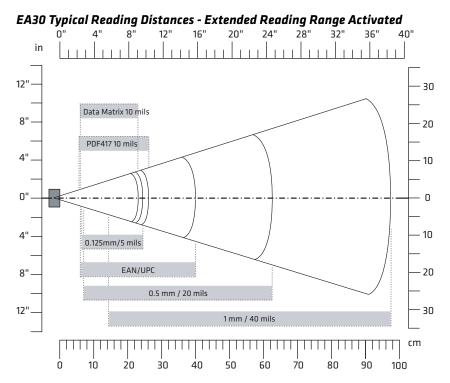
EA30 Typical Reading Distances - Extended Reading Range Activated
