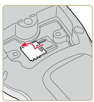
**5** Slide the microSD card door towards the top of the computer to unlock it and open the door.
