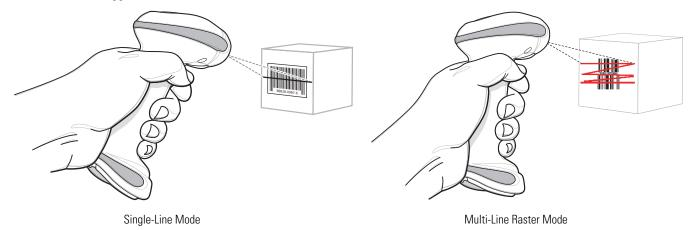
Figure 2-1. Scanning in Hand-Held Mode
