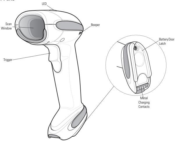
Figure 1-2. Parts of the Scanner
