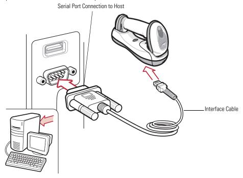
Figure 7-1. RS-232 Direct Connection
