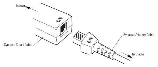
Figure 1-6. Synapse Cable Connection
