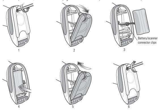
Figure 1-7. Inserting the Battery
