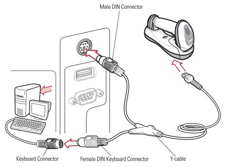
Figure 6-1. Keyboard Wedge Connection with Y-cable
