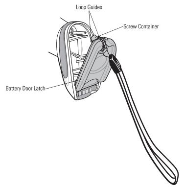
Figure 1-11. Attaching Lanyard
