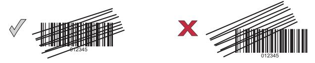
Figure 2-3. Acceptable and Incorrect Multi-Line Aiming
