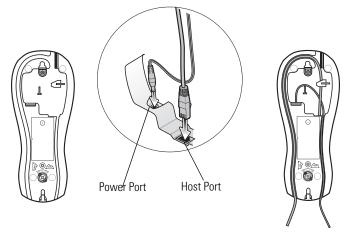
Figure 1-5. Connecting the Cables to the Cradle
