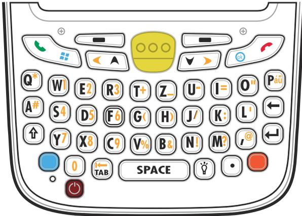
Figure B-4 QWERTZ Keypad Configuration
