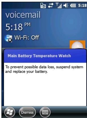
**Figure 2-21** Main Battery Temperature Watch Dialog Box
