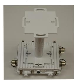
4. With the Access Point positioned so that the gore vent is facing down, attach the extension arm to the Access Point bracket section with two ½ inch bolts and nuts. Tighten bolts to 300 inch pounds (lbf-in).
