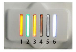
The Access Point utilizes two different colored lights below each LED. Only one light displays within an LED at any given time. Every light within each LED is exercised during startup to allow the user to see if an LED is not functioning. The LEDs turn on and off while rotating in a circular pattern. Since two LEDs feed each light pipe, the pattern is from left to right (LEDs 1 through 6), then right to left (LEDs 6 through 1).
