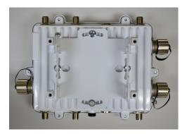
5. Insert two M6 hex flange screws into the bottom holes on the sides of the Access Point bracket section.
