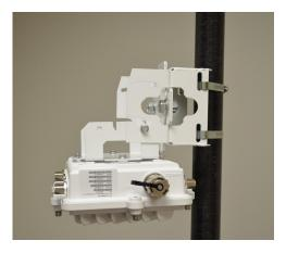
6. Rotate the Access Point bracket section upward and align the top holes on the sides with the top holes on the angle adapter bracket section. Insert two M6 hex flange screws into the top holes on the angle adapter bracket section.
