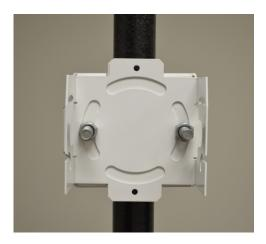
4. Position the Access Point bracket section so that the bottom of the section with the straight (not bevel cut) side is oriented toward the bottom side of the AP with the gore vent. Using a torque wrench or a ratchet and a 10mm socket, or an adjustable wrench, attach (but don't tighten) the Access Point bracket section to the AP 7161 with the four M6 flange screws
