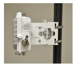
7. Use a torque wrench or a ratchet and a 10mm socket, or an adjustable wrench, to finish attaching the Access Point bracket section to the angle adapter bracket section with the M6 hex flange screws in the open slot connections and the top holes on the angle adapter bracket section. Do not tighten the screws until all rotation and tilt adjustments are complete.
