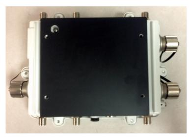
3. Put the chassis mount on the flat plate with the key hole and four screw holes aligned.
