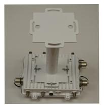
4. With the Access Point positioned so that the gore vent is facing down, attach the extension arm to the Access Point bracket section with two 1/2 inch bolts and nuts. Tighten the nuts to 30 inch pounds (lbf-in).
