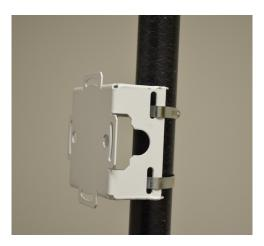
2. With the angle adapter bracket section positioned so that the open connector slots are on the bottom, attach the angle adapter bracket section to the pole mount bracket section using two 1/2 inch bolts and nuts. Tighten the nuts to 30 inch pounds (lbf-in).
