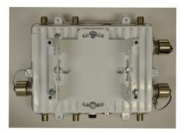
6. With the Access Point positioned so that the gore vent is facing down, insert the two M6 hex flange screws in the bottom holes on the sides of the Access Point bracket section into the open slot connections on the bottom of the angle adapter bracket section.
