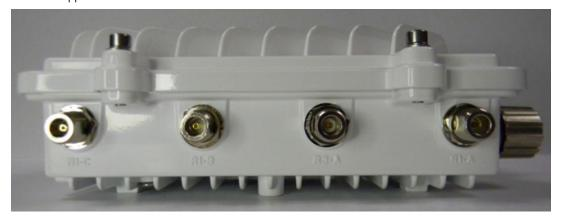
As with the two radio models, R1 ports relate to the software configured radio 1 settings. When mounting antennas to connectors marked R2-A, R2-B and R2-C, the antenna ports relate to the software configured radio 2 settings. Care must be taken to provide the correct antenna for the operating band of each port.
