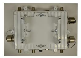
3. With the Access Point positioned so that the gore vent is facing down, insert the two M6 hex flange screws in the bottom holes on the sides of the Access Point bracket section into the open slot connections on the bottom of the angle adapter bracket section. Rotate the Access Point bracket section upward and
