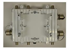
5. With the Access Point positioned so that the gore vent is facing down, insert the two M6 hex flange screws in the bottom holes on the sides of the Access Point bracket section into the open slot connections on the bottom of the angle adapter bracket section.
