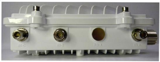
When mounting antennas to ports R1-A, R1-B, and R1-C, ensure that you have selected the appropriate band for the configured radio that uses ports R1-A, R1-B, and R1-C. In this instance, R1 ports relate to the software configured radio 1 settings.
