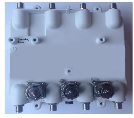
The grounding post is located on the bottom of the Access Point above the GND symbol.
