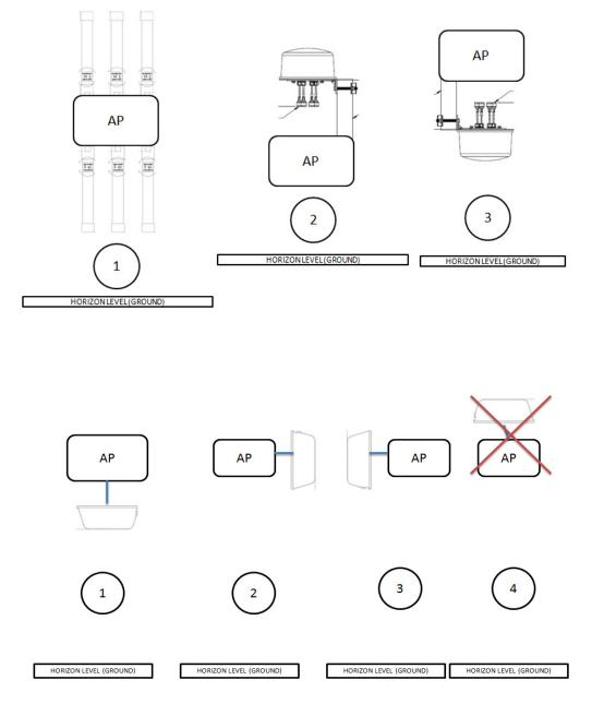
For the units utilizing an antenna façade, the unit can be mounted on a pole or in the ceiling as long as the unit faces its intended radio coverage area.
