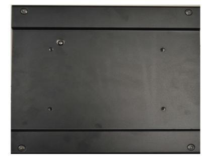
3 Put the chassis mount on the flat plate with the key hole and four screw holes aligned.
