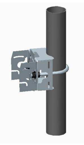
3 Place the angle adapter bracket on the U-bolt with the open slot connections on the bottom and align it with the pole mount. Attach with two 1/2 inch nuts. Tighten all nuts to 300 inch pounds (lbf-in).
