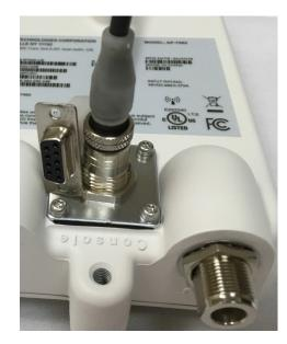
*Pin 1* - Transmit from Access Point *Pin 2* - Receive to Access Point *Pin 3* - Ground
