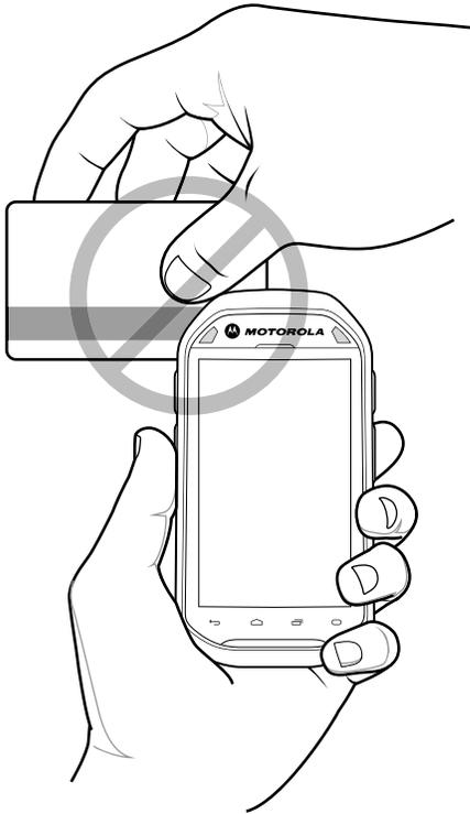
**Figure 3-8 Do Not Hold End of Card While Swiping**
