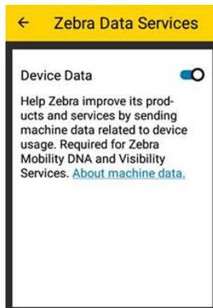
Touch the **Device Data** switch to disable the device from sending analytics data. Zebra recommends keeping this option enabled.
