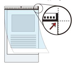
3 Load the Carrier Sheet in the ADF paper chute.
