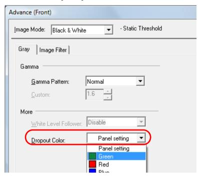
If you select [Panel setting], the setting of the Software Operation Panel is enabled.
