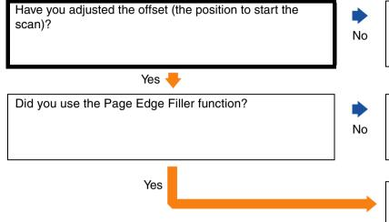
Go to [Device Setting] of the Software Operation Panel, and adjust the offset in the sub-scanning direction.
