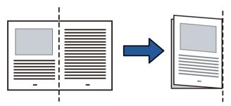
2 Place the document inside the Carrier Sheet. Align the fold line with the right edge of the Carrier Sheet so that the document fits in the upper right-hand corner.
