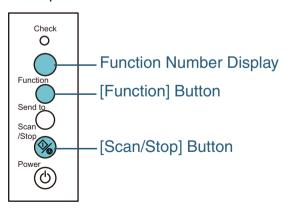
Press the [Function] button and confirm that the function number is flashing faster, then either press the [Scan/Stop] button or perform a scan from the computer.
