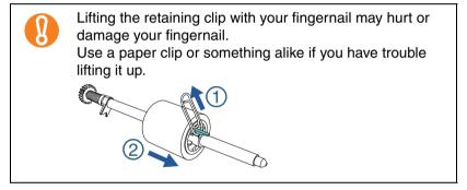
8 Attach a new pick roller on the shaft.
