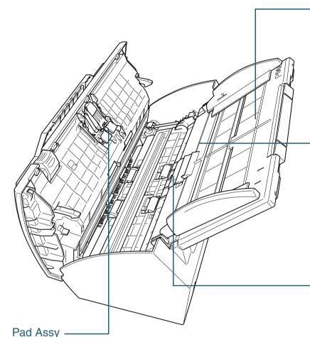
For details about removing the pad assy, refer to "7.2 Replacing the Pad Assy" (page 96).
