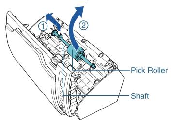
The area around the pick roller may be contaminated by paper dust which can cause scanning errors. Wipe off the paper dust with a cloth moistened with Cleaner F1.
