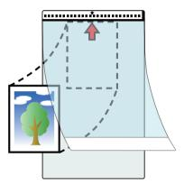
2 Load the Carrier Sheet face-down in the ADF paper chute, as shown below.
