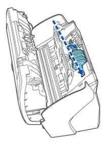
2) Rotate the Pick roller lever in the direction of the arrow.
