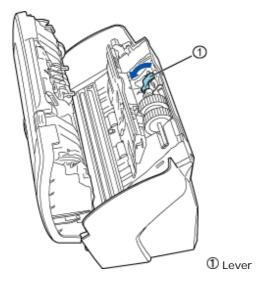
3) Slide the Pick roller in the direction of teh arrow, and then lift it up to remove the shaft from the hole.
