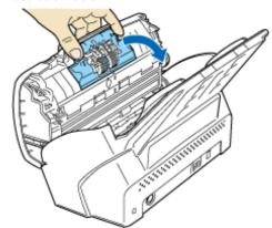
2) Lift up the right side of the Brake roller and remove the right side of the shaft. Then pull the left side of the shaft out of its hole to remove it.
