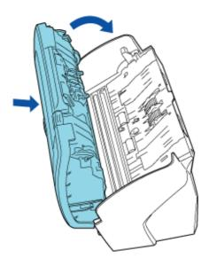
9. Attach the ADF paper chute to the scanner.
