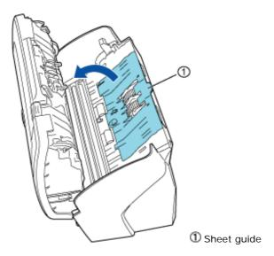
2) Rotate the Pick roller lever in the direction of the arrow.
