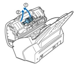
4. Remove the Brake roller from the shaft.
