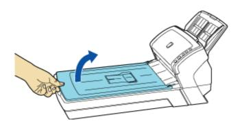
2. Load the document on the document bed with the scanning face down and the top left corner aligned with the reference point (1).
