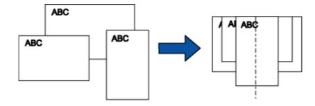
3. Place the documents on the ADF paper chute, and then adjust the side guides so that they lightly touch the widest sheets of paper.
