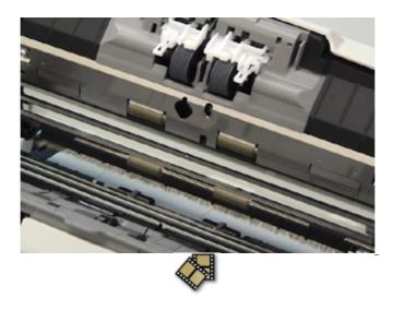
3. Press down on the center of the ADF to return it to its original position until the ADF button locks.
