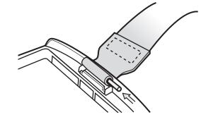
Figure 1-15 Feed handstrap into Handstrap Slot
