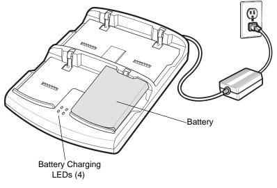
Figure 6-10 Four Slot Battery Charger
