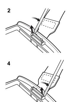
Figure 1-13 Handstrap and Pin Removal
