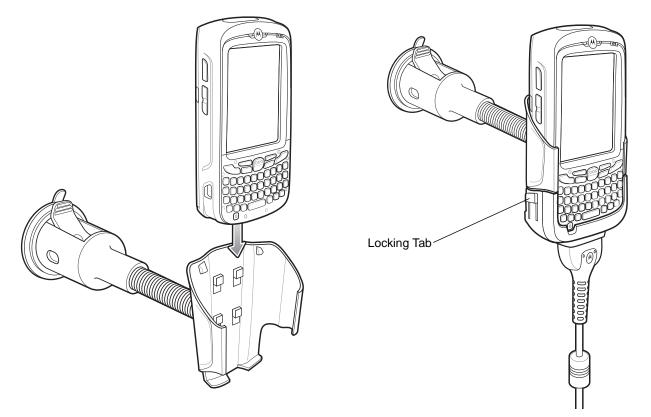
Figure 6-14 Insert MC55 into Vehicle Holder
