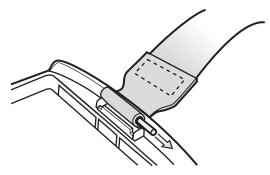
Figure 1-14 Pin Removal
