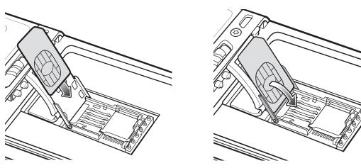
Figure 1-6 Inserting the SIM Card
