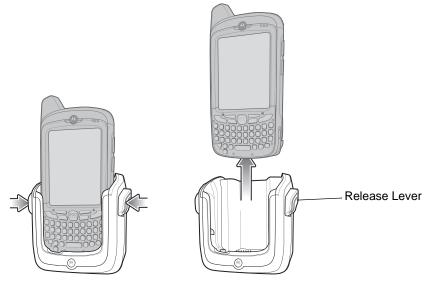
Figure 6-9 Removing the MC55
