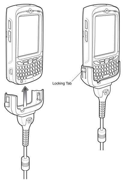
Figure 6-11 Cable Cup Locking Tabs
