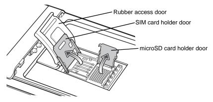
Figure 1-3 Lift SIM Slot Holder Door
