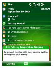
Figure 2-9 Main Battery Temperature Warning Dialog Box
