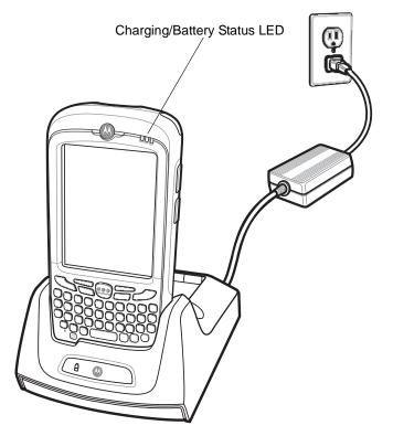
Figure 6-1 MC55 Battery Charging
