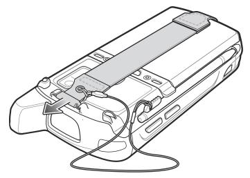
Figure 1-12 Handstrap Clip Removal
