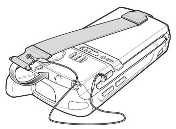
Figure 1-17 Slide Handstrap and Tether Over Handstrap Mount
