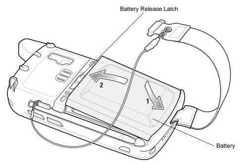
Figure 1-7 Inserting the Battery
