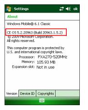
The second line lists the operating system version and the build number. The last part of the build number represents the AKU number. For example, *Build 20963.1.5.2* indicates that the device is running AKU version *1.5.2*.
