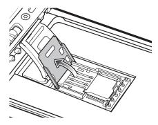
Figure 1-5 Lifting the SIM Cover
