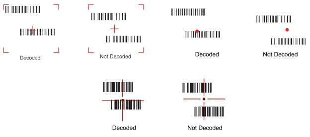
Figure 2-28 Pick List Mode with Multiple Bar Codes in Aiming Pattern
