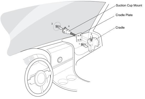
Figure 6-13 Windshield Installation
