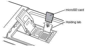
Figure 1-4 Insert microSD Card in Holder
