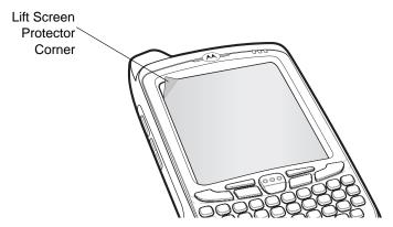
Figure 7-1 Removing the Screen Protector
