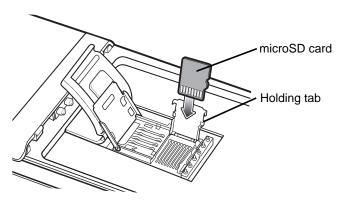
Figure 1-2 Insert microSD Card in Holder
