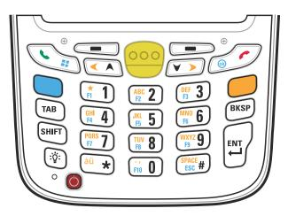
Figure B-1 MC67 Numeric Keypad
