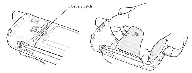
Figure 1-6 Removing the Battery
