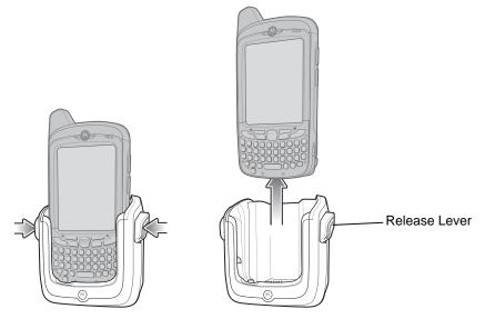
Figure 10-10 Removing the MC67
