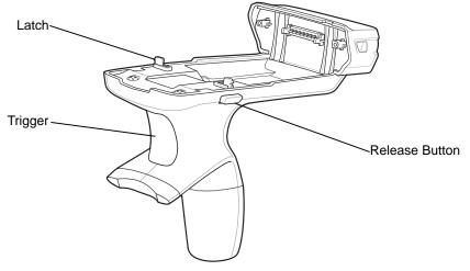
Figure 10-13 Trigger Handle Features
