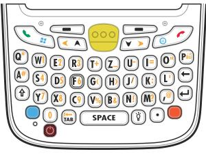
Figure B-4 QWERTZ Keypad Configuration
