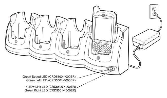
Figure 10-7 MC67 Battery Charging
