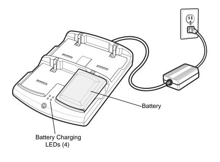
Figure 10-11 Four Slot Battery Charger
