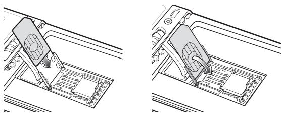
Figure 1-4 Inserting the SIM Card
