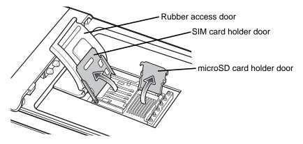
Figure 1-1 Lift SIM Slot Holder Door
