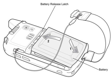
Figure 1-5 Inserting the Battery
