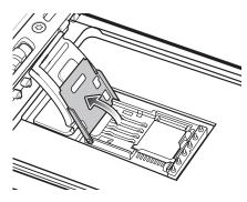
Figure 1-3 Lifting the SIM Cover
