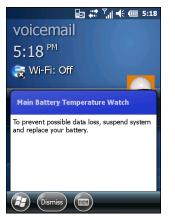
Figure 2-21 Main Battery Temperature Watch Dialog Box
