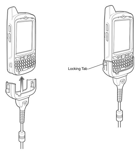
Figure 10-12 Cable Cup Locking Tabs
