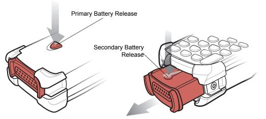
Figure 1-6 Removing the Main Battery - MC909X-S
