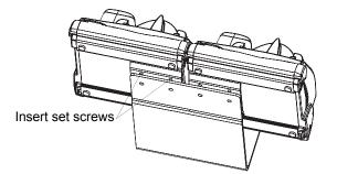
Figure 2-66 Attaching Two Shelf Slides
