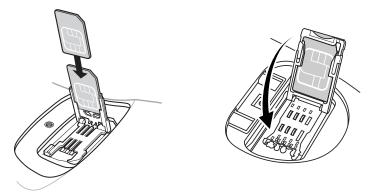
Figure 1-10 Inserting the SIM Card
