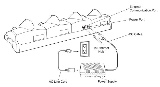
Figure 2-9 Four Slot Ethernet Cradle Power Connection
