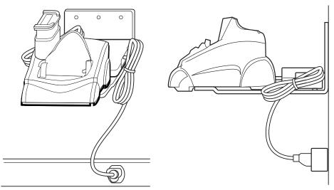
Figure 2-61 Mounted Single Slot Cradle With Power Connection
