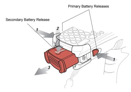
Figure 1-5 Removing the Main Battery
