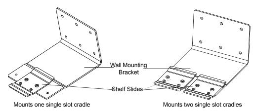
Figure 2-60 Wall Mounting Bracket with Shelf Slide
