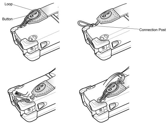
Figure 1-14 Repositioning the MC909X-K Strap
