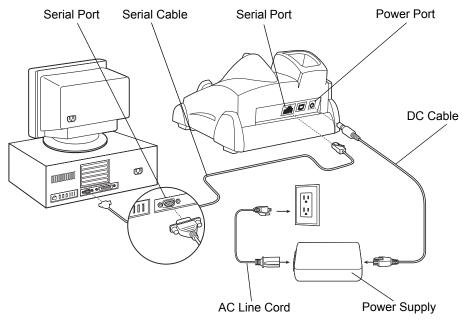
Figure 2-6 Single Slot Cradle Power/Serial Connections
