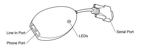
Figure 2-30 Modem Module
