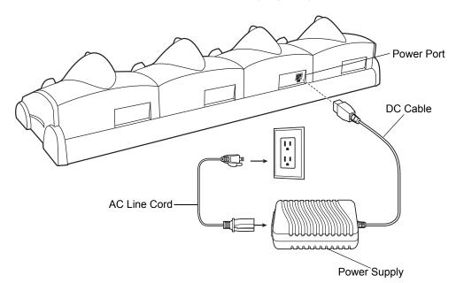
Figure 2-15 Four Slot Charge Only Cradle Power Connection
