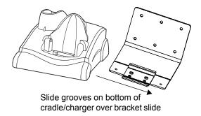
Figure 2-65 Attaching Two Shelf Slides
