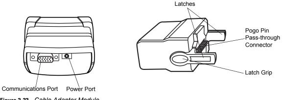
Figure 2-23 Cable Adapter Module
