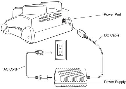
Figure 2-17 Four Slot Spare Battery Charger Power Connection
