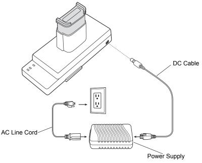
Figure 2-28 UBC Adapter Power Connection
