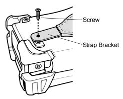
Figure 1-16 Repositioning the MC909X-S Strap
