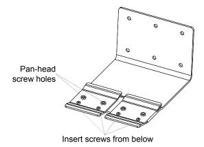
Figure 2-64 Attaching Two Shelf Slides
