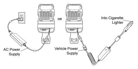
Figure 2-25 CAM Power Connection
