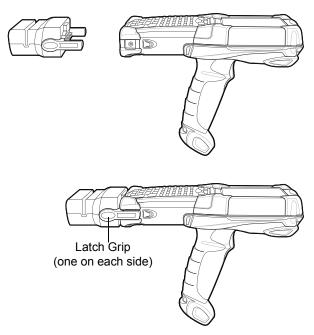
Figure 2-19 Attaching the MSR
