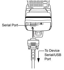
Figure 2-21 MSR Serial/USB Connection
