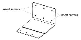
Figure 2-62 Wall Mounting Bracket Mounting Screws
