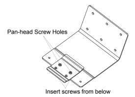
Figure 2-63 Attaching One Shelf Slide
