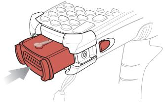
Figure 1-4 Installing the Main Battery
