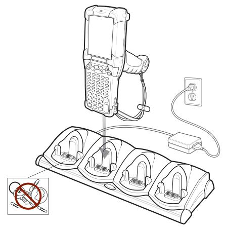
Figure 2-14 Four Slot Charge Only Cradle
