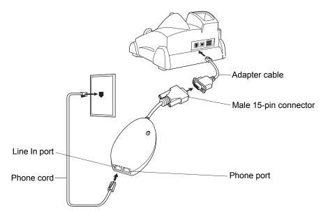
**Connecting to the Single Slot Serial/USB Cradle**
