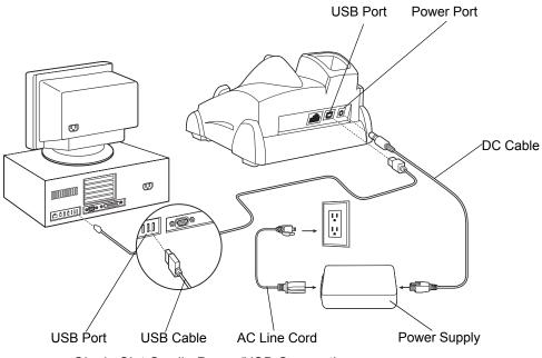
Figure 2-7 Single Slot Cradle Power/USB Connections
