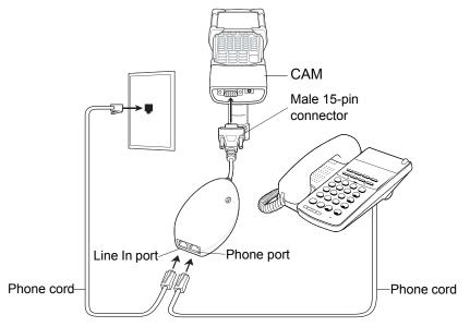
Figure 2-31 Modem Module Connection - Mobile Computer
