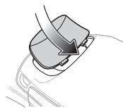
Figure 1-12 Replacing the SIM Door
