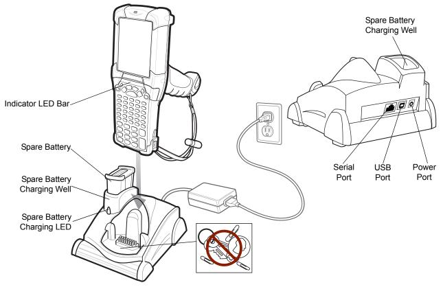
Figure 2-4 Single Slot Serial/USB Cradle
