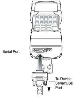
Figure 2-26 CAM Serial Connection
