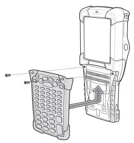
Figure 2-2 Installing the Keypad
