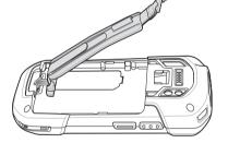
3. Insert the bottom of the battery into the battery compartment.
