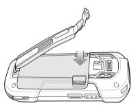
5. Place the hand strap clip into the hand strap attachment slot and pull down to lock into place.
