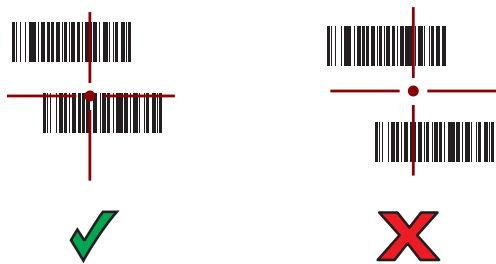
Figure 4-3 Pick List Mode with Multiple Bar Codes in Aiming Pattern
