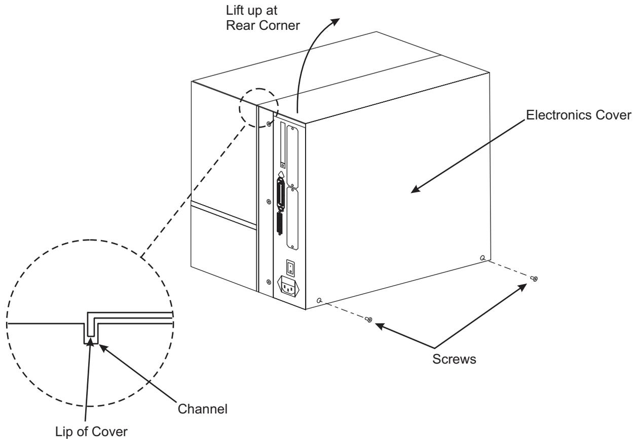
**Figure 4-9. Removing and Installing the Electronics Cover**
