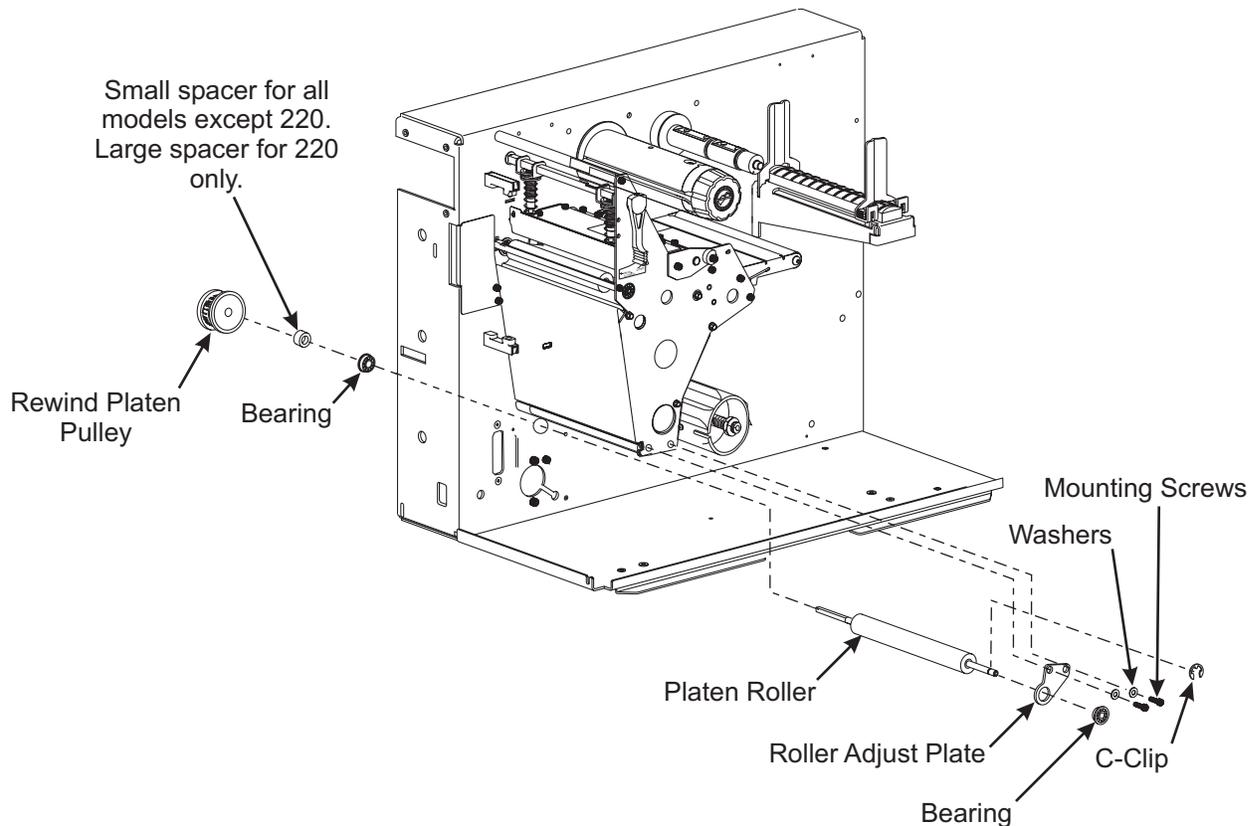
**Figure 4-33. Print Mechanism View with Lower Platen Roller**
