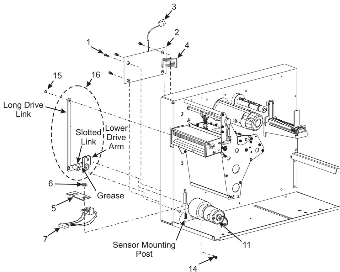
**Figure 6-35. Linkage and Circuit Board Installation**
