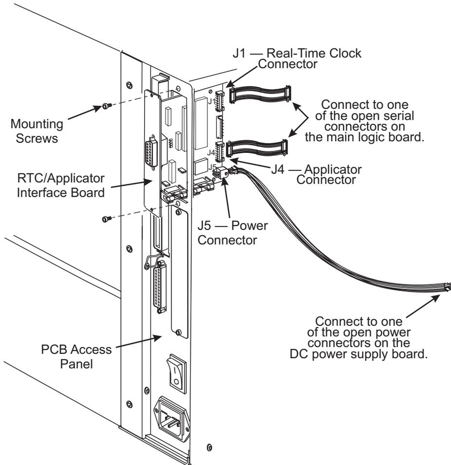
**Figure 6-30. Applicator/Real-Time Clock Installation**
