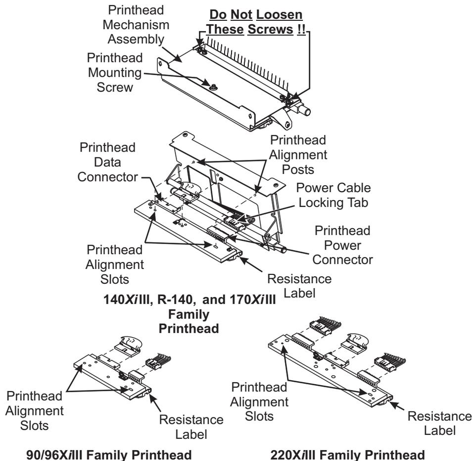
**Figure 4-22. Printhead Replacement**
