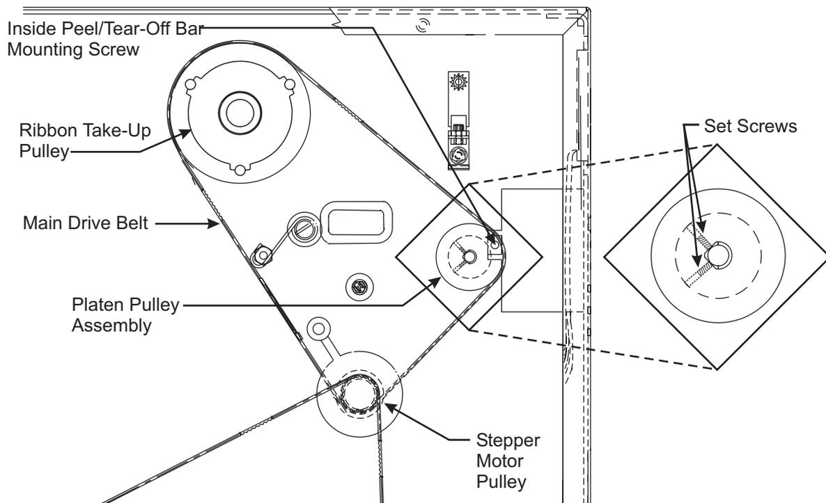
**Figure 4-35. Platen Pulley Replacement**
