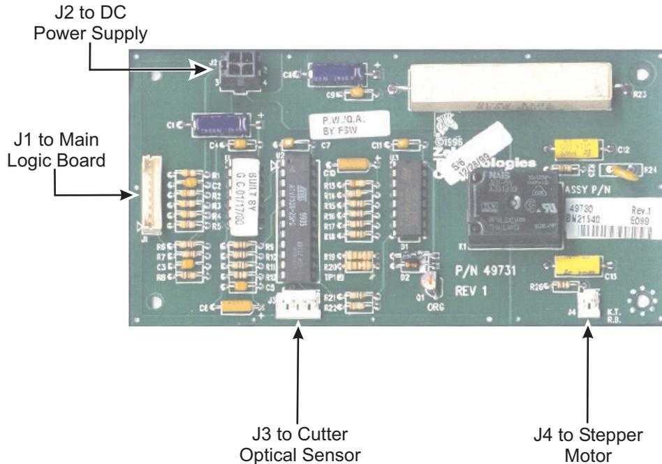
**Figure 6-37. Cutter Option Circuit Board**
