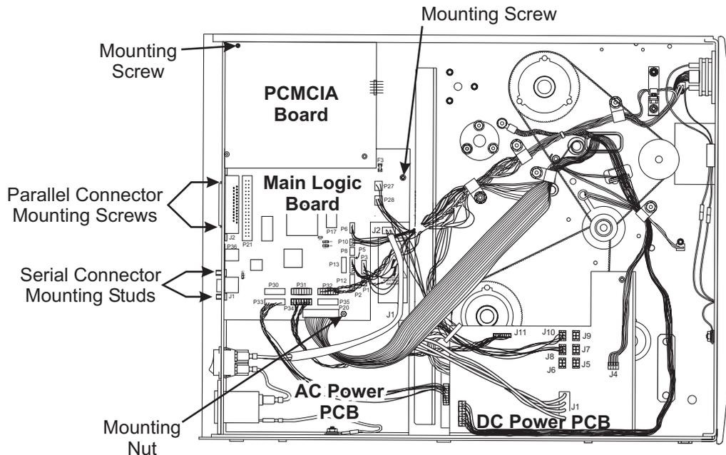
**Figure 4-15. PCMCIA and Main Logic Board Removal and Installation**
