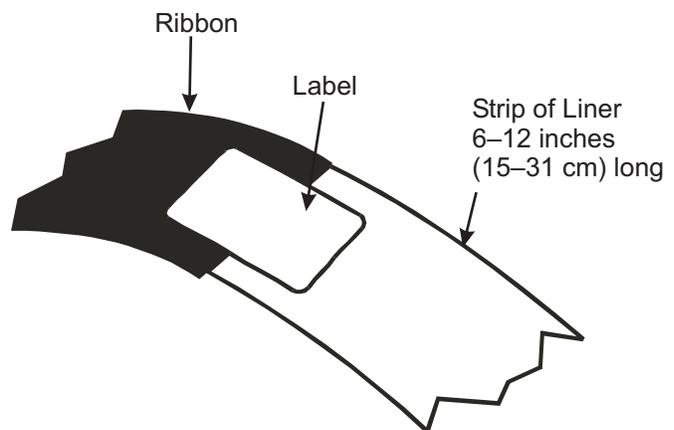
5. Thread the ribbon (with leader, if used) as shown in Figure 2-11 without creasing or wrinkling it.
