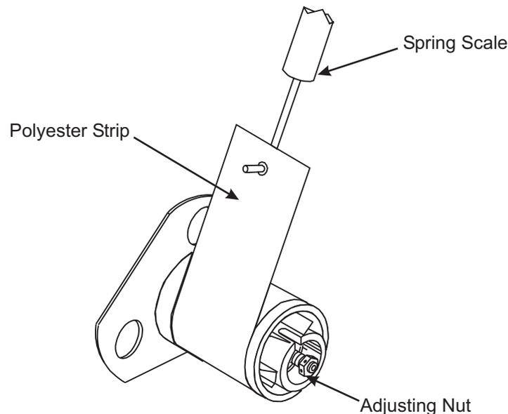
**Figure 6-13. Tension Adjustment of Rewind Spindle Assembly**
