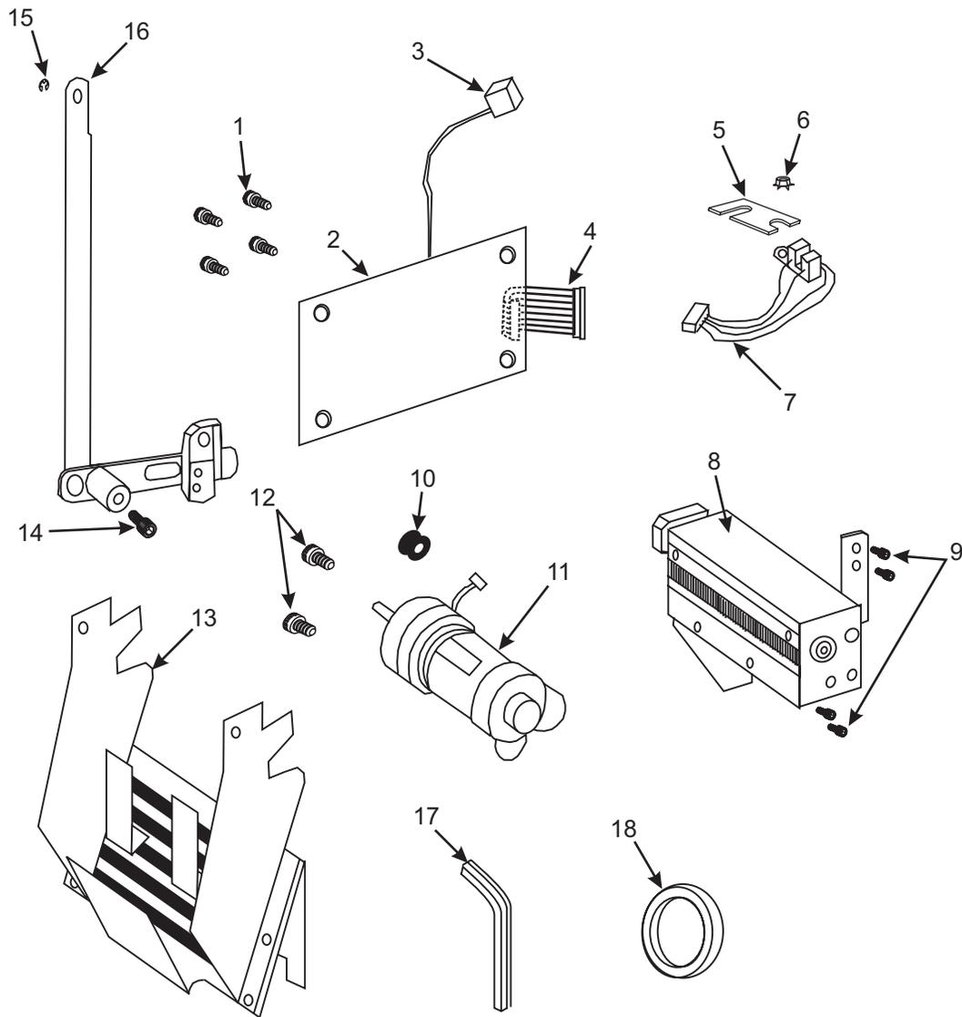
**Figure 6-31. Part Identification Cutter Option**
