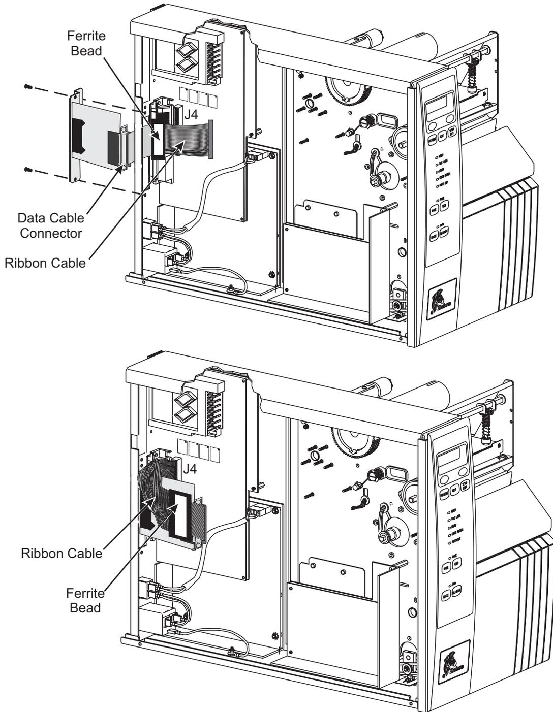
**Figure 6-17. X1111 and R-140 Internal PrintServer II Board Installation**
