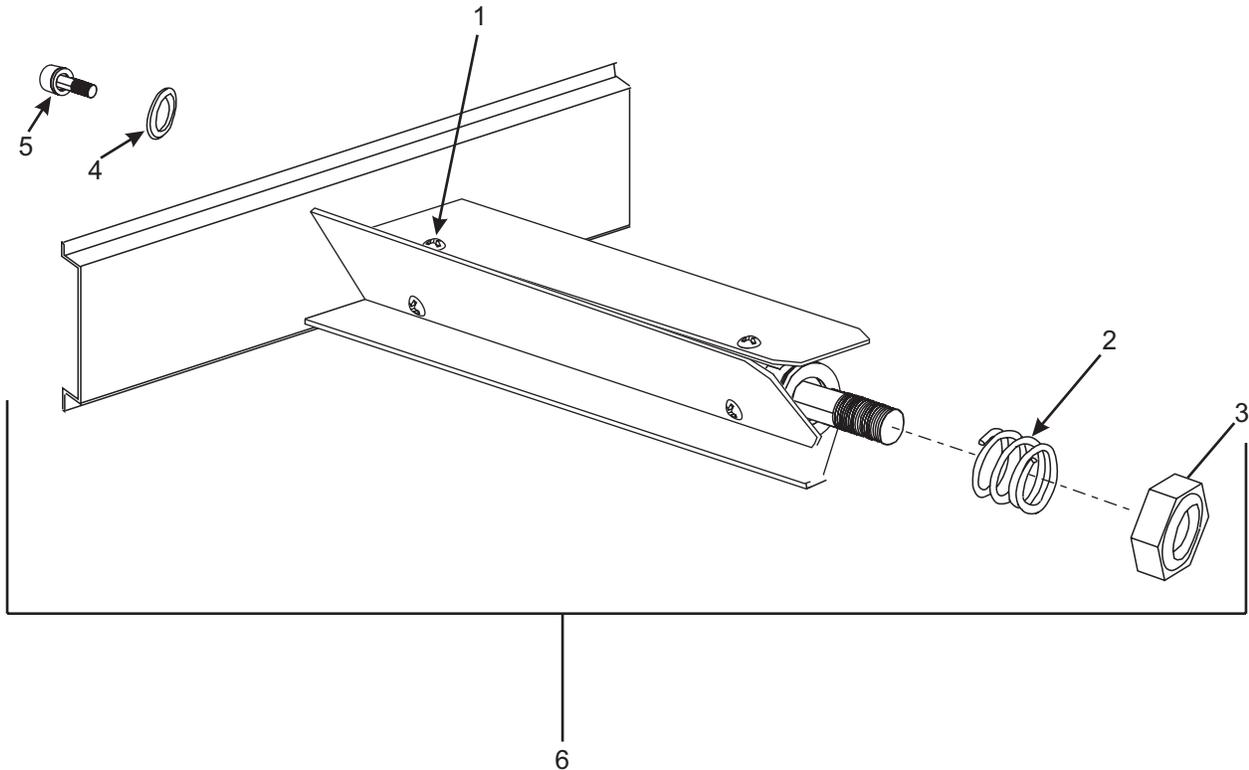
**Figure 5-14. Optional Media Supply Spindle**
