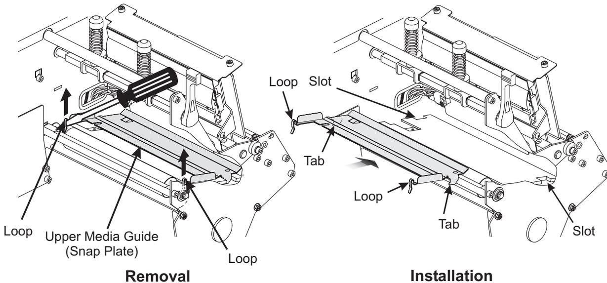
**Figure 4-2. Current Snap Plate Removal and Installation**
