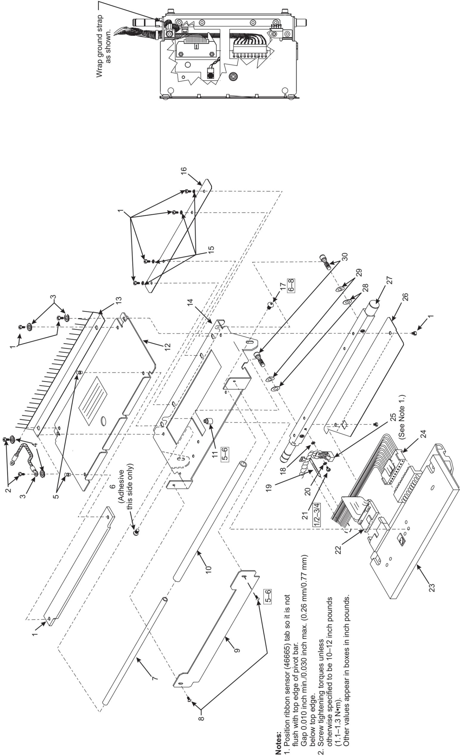
**Figure 5-11. Printhead Support Assembly 90/96X/III, 140X/III, and 170X/III**
