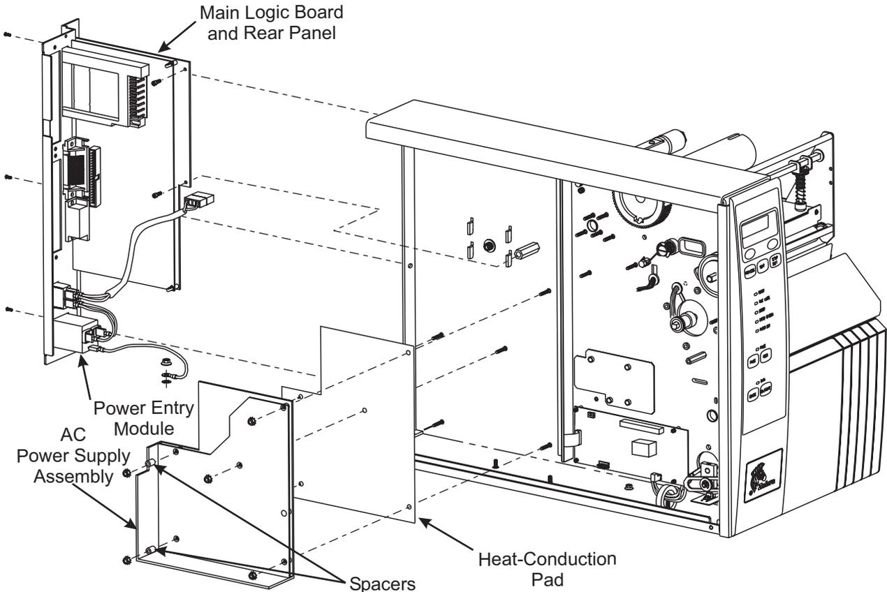
**Figure 4-16. AC Power Supply and Main Logic Board Removal/Installation**
