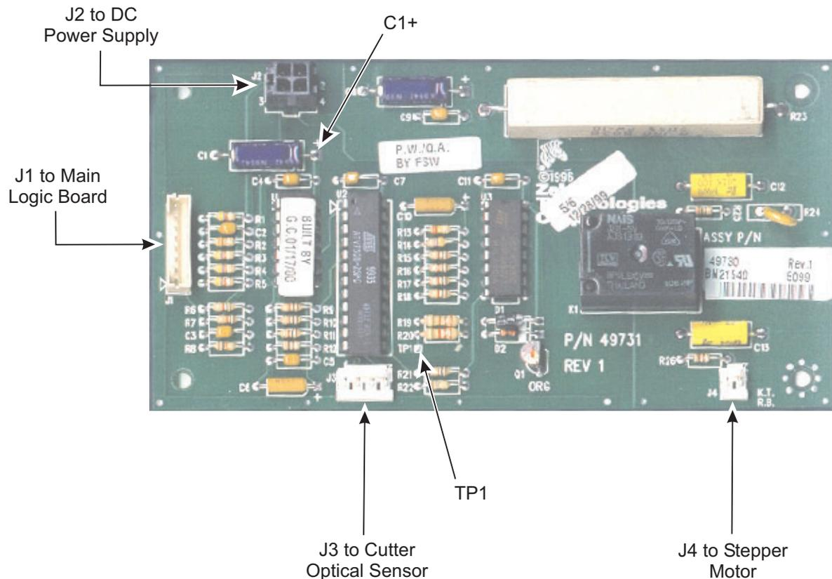
**Figure 4-40. Cutter PCB Connections**
