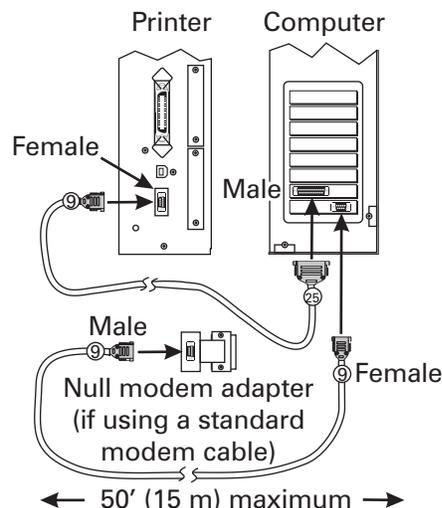
**Figure 1-6. Serial Data Port**
