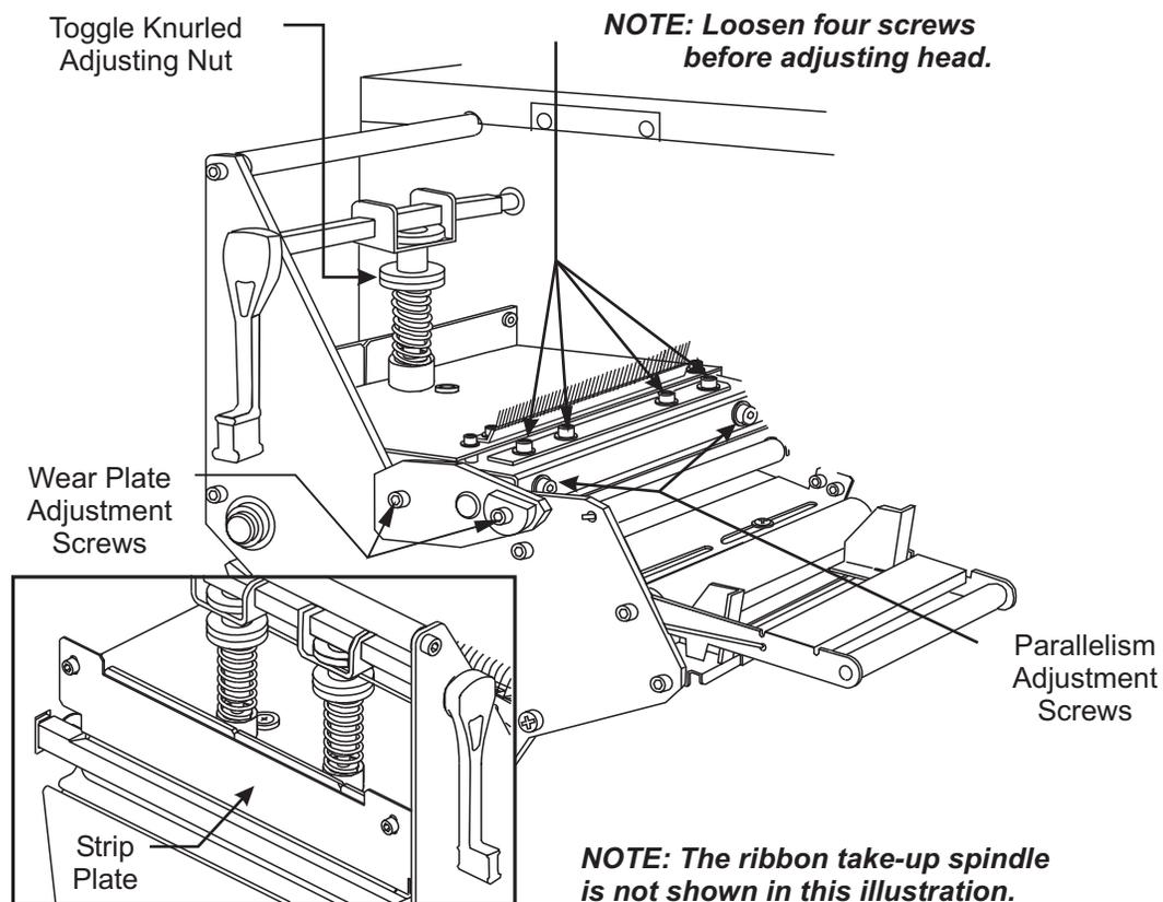
**Figure 4-24. Printhead Adjustment**
