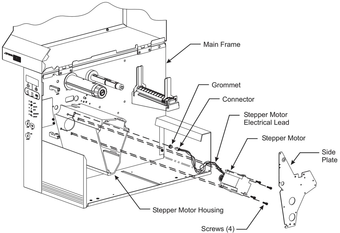
**Figure 4-58. DC Stepper Motor Removal and Installation**
