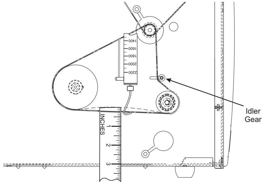
**Figure 4-19. Rewind Drive Belt Tension Adjustment**
