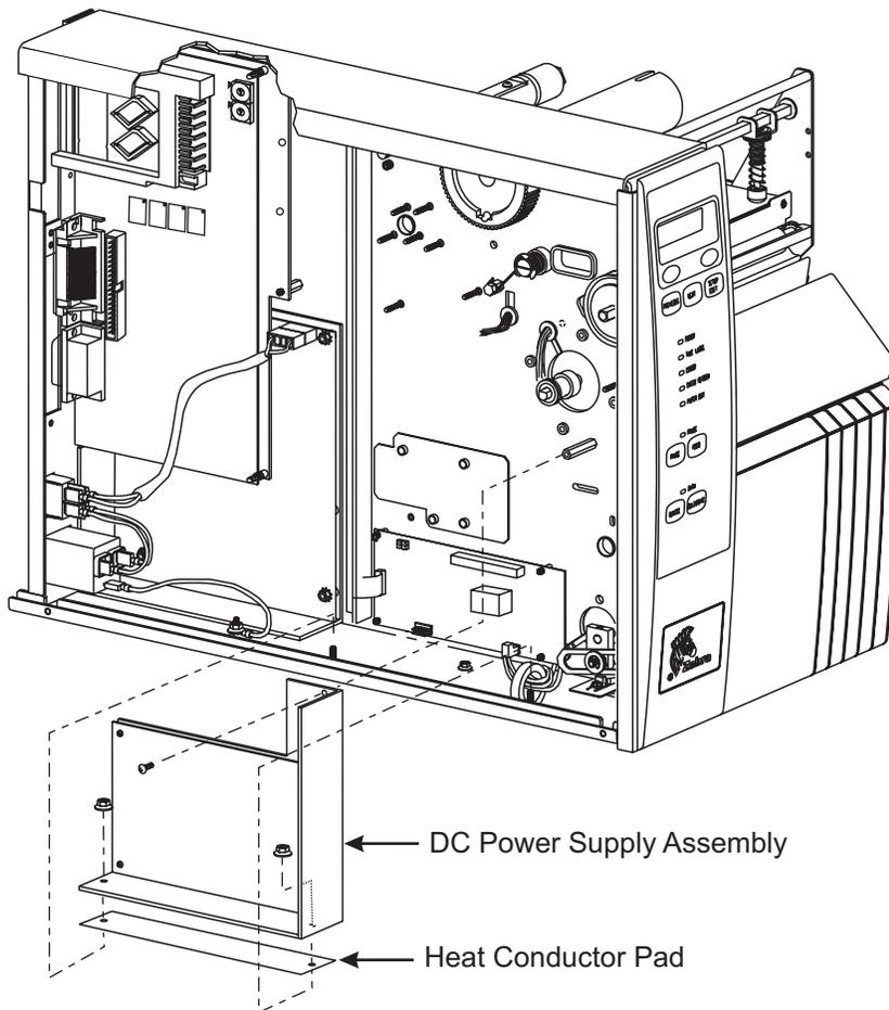
**Figure 4-10. DC Power Supply Removal and Installation**
