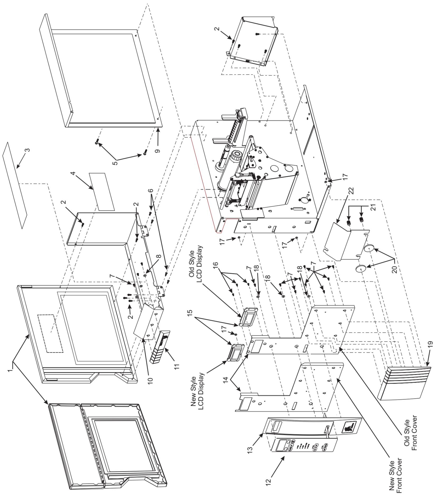
Figure 5-1. Final Assembly 90/96/140/170XIII/XIIIPlus and R-140 Mechanical
