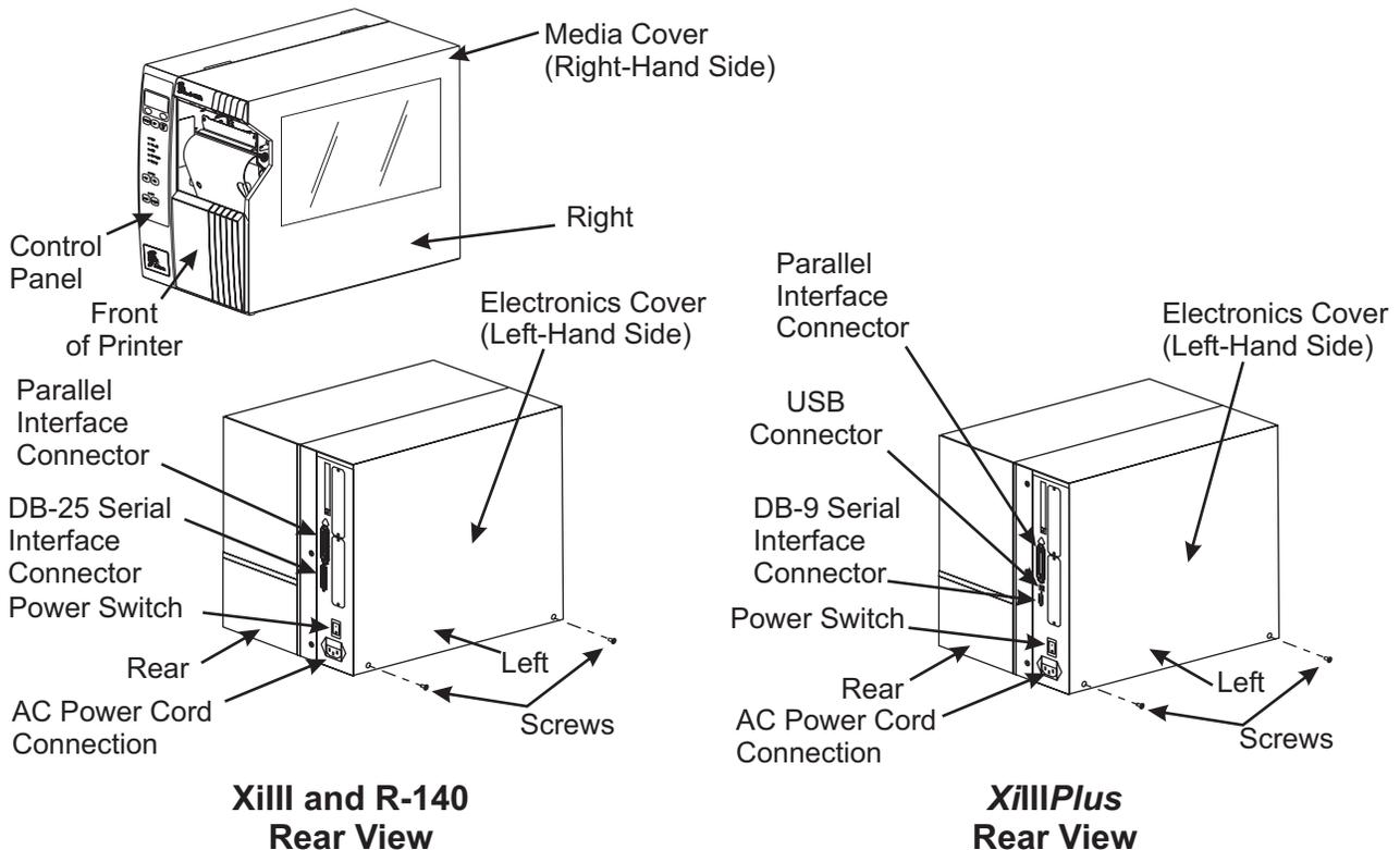
**Figure 4-4. External Printer Components Orientation**
