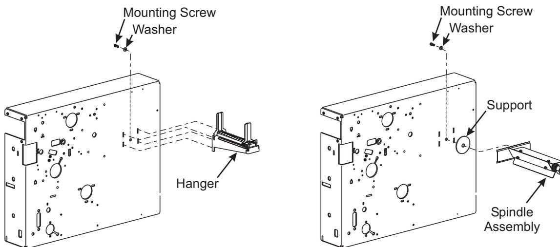
**Figure 6-5. Hanger Removal and Spindle Installation**
