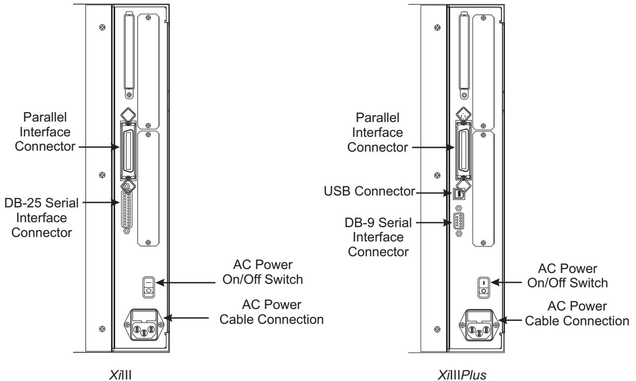
**Figure 1-4. Interface Connections**
