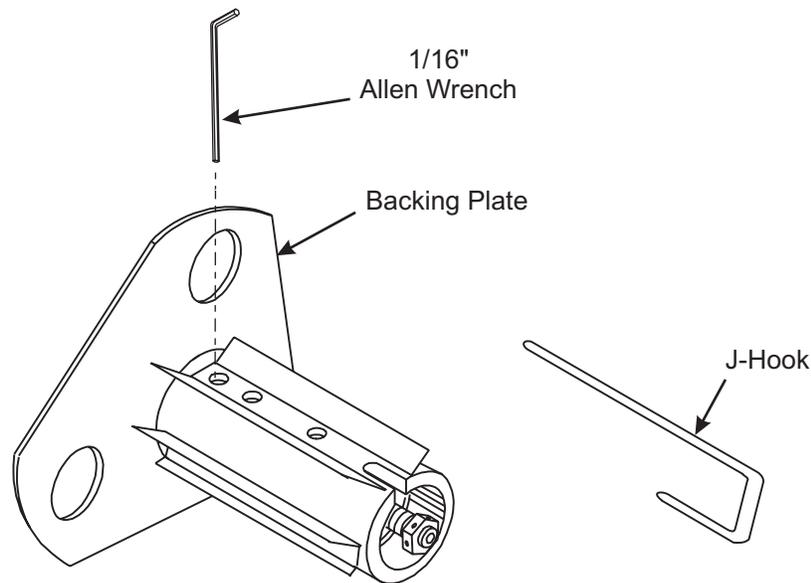
**Figure 6-12. Position Adjustment of Rewind Spindle Assembly**
