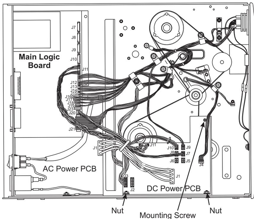
**Figure 6-32. DC Power PCB Location and Interconnections**
