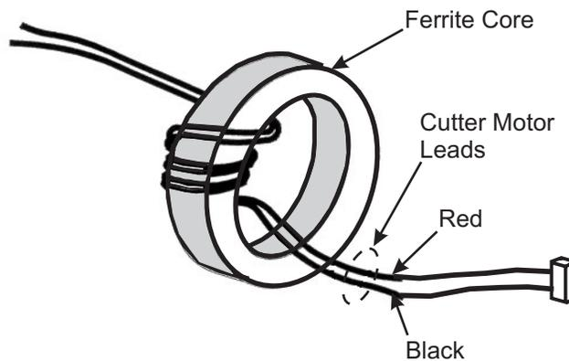
**Figure 6-38. Cutter Motor Leads**
