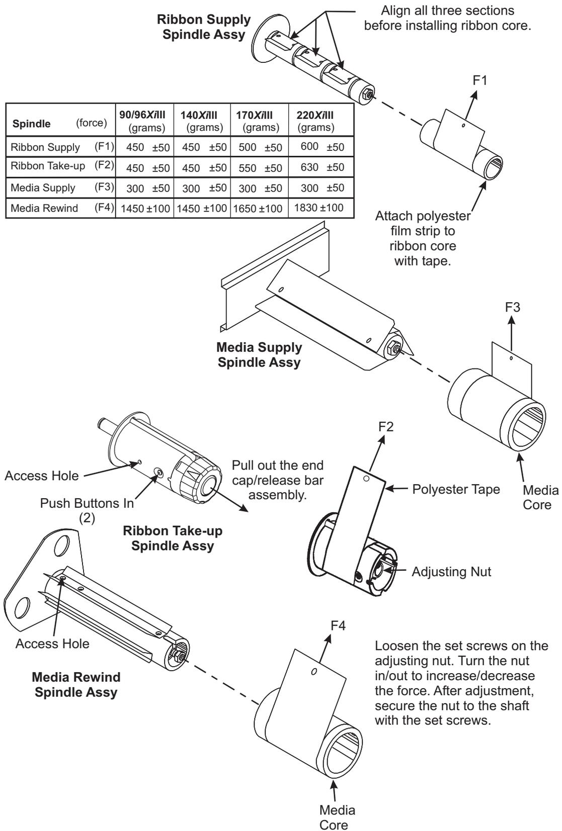
**Figure 4-29. Spindle Tension Adjustments**
