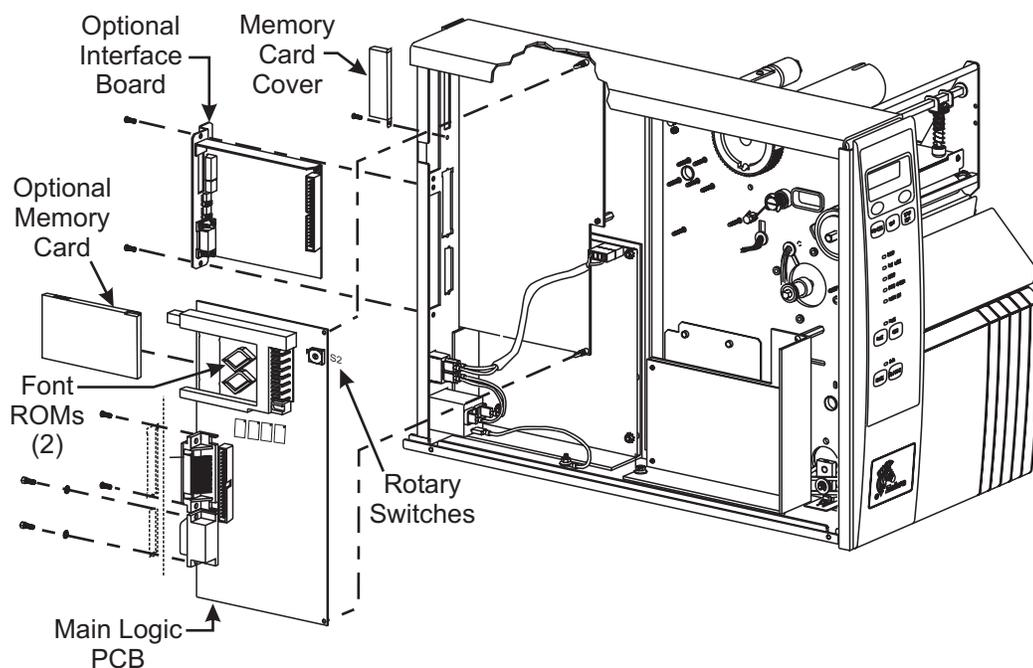
**Figure 4-11. Main Logic Board Removal and Installation**
