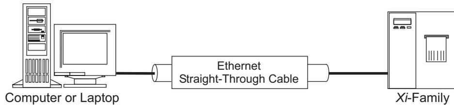
**Figure 6-26. Straight-Through Cable Environment**
