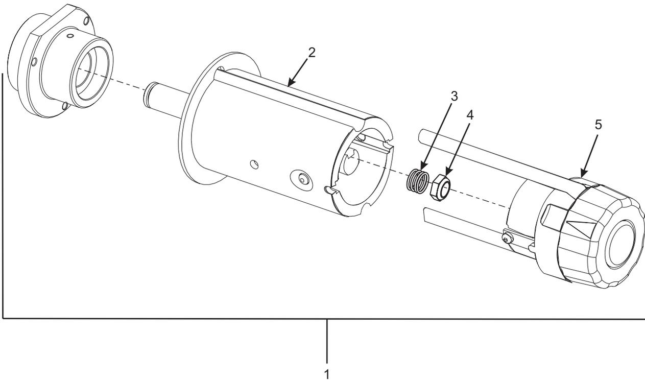
**Figure 5-16. Ribbon Take-Up Spindle Assembly**
