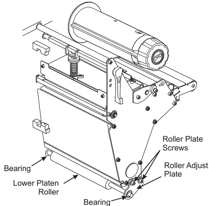
**Figure 4-34. Peel-Off Lower Roller Alignment**
