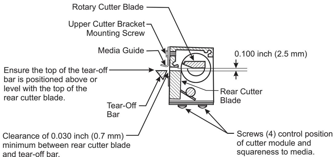
Relative position of the rotary cutter blade when the drive link assembly is stopped by the optical sensor, when power is on in the cutter mode.
