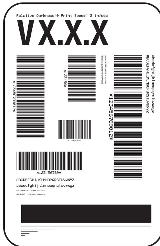
Figure 3-3. FEED Key Self Test Sample Label
